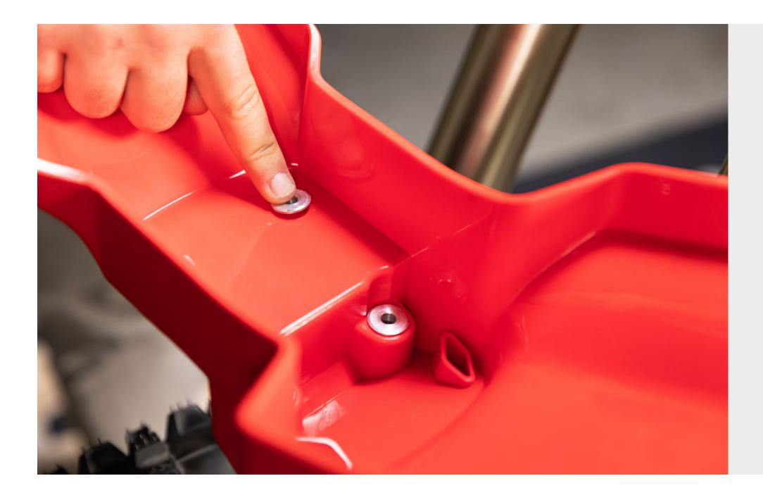
32 Place the front fender in between the fork and align the notches in the front fender with the fastening points in the frame.
