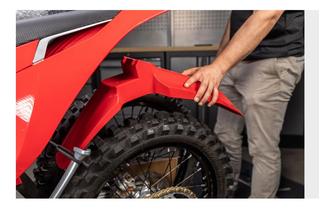
Unscrew the number plate and 5 remove it from the motorcycle.
