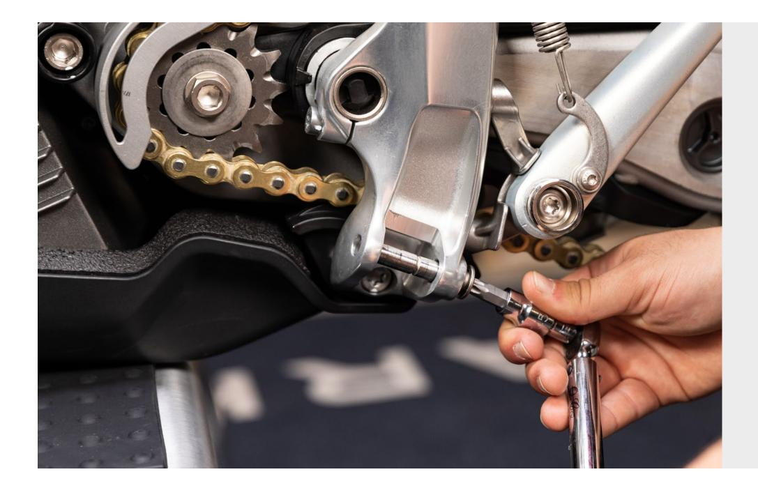
37 Place the left foot peg inside the recess on the left side of the motorcycle and gently push the **foot peg** inside the recess to align the shaft.
