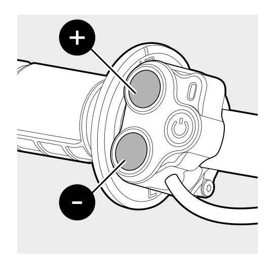
Press the **+ button** once to move up one ride mode. Press the **- button** once to move down one ride mode.
