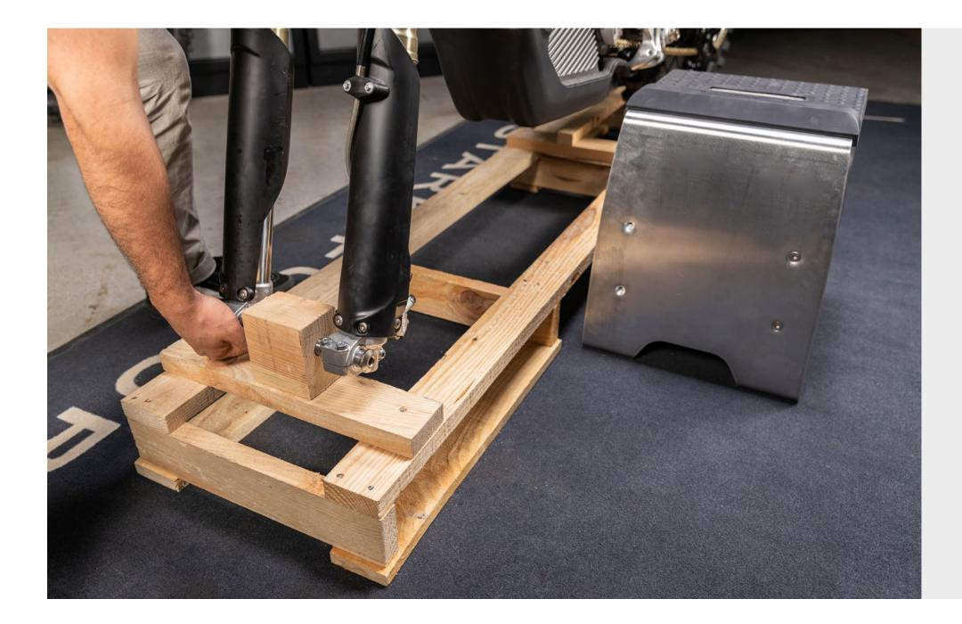
22 Lift and turn the back of the **frame** until the skid plate is in the center of the charger stand and the motorcycle is evenly balanced.
