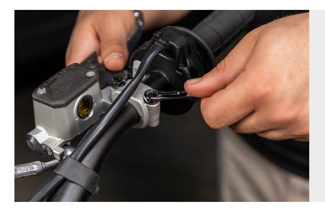
**11** If your bike is equipped with rear hand brake instead of rear foot brake, repeat the provious stop to attach the **rear hand**
